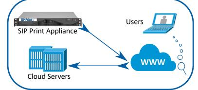
When a User plays a call, the media file is pushed from the premise based SIP Print Appliance over a secure (SSL) connection to the SIP Print Cloud Servers then down to the Users Web client.
