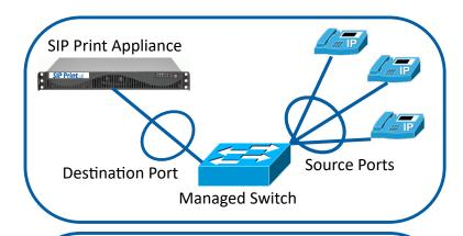
Meta data is pushed to the SIP Print Cloud over a secure Outbound Connection to NIST compliant servers where the call records are searchable in the SIP **Print Cloud Portal**
